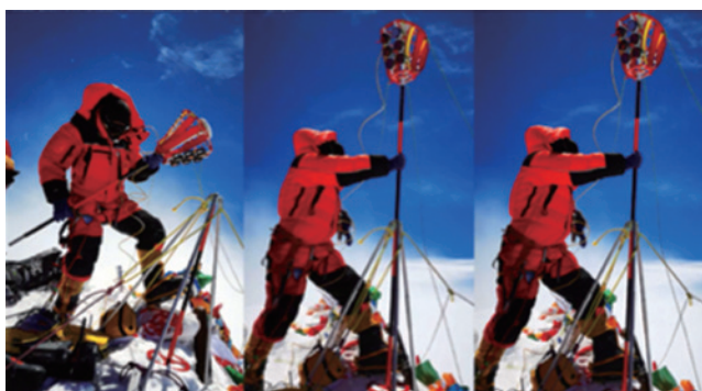
Setting up the remote target at the summit of Mount Everest. (Photo: Xinhua)
