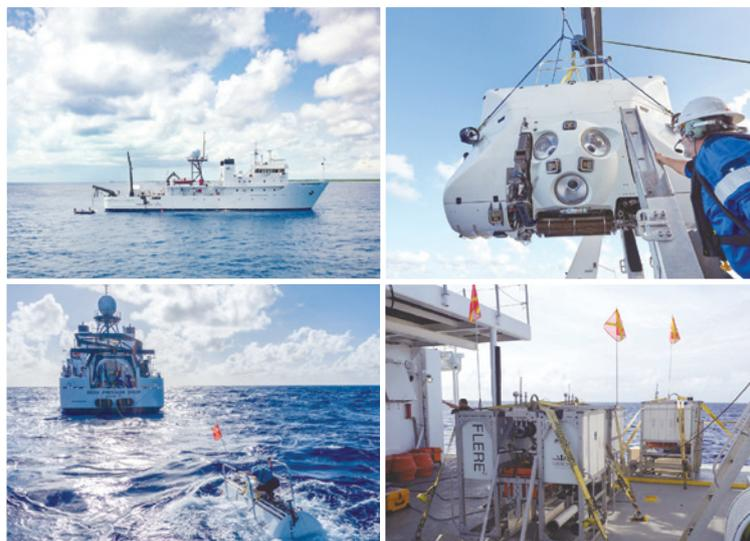
*Limiting Factor*, a Triton (Submarines) Model 36000/2 submersible, remains the centrepiece of the system. It is named for its full-ocean depth certification and crew capacity of two. For a submersible, it is compact (4.6 X 1.9 X 3.7 metres), lightweight, and designed to travel vertically through the water column as quickly as possible at speeds of up to 3.5 knots vertically or 2-3 knots laterally at depth.
