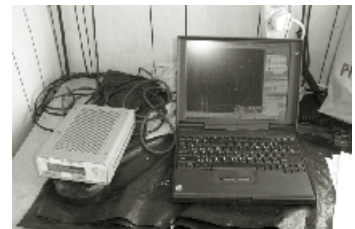
Figure 4: Seastar 3000L receiver and the real-time data processing computer
