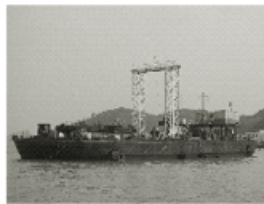
Figure 2: A 165-foot long "Standpiper" Drilling Barge
