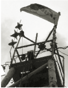
Figure 5: Seastar beacon antenna is mounted on top of a barge
