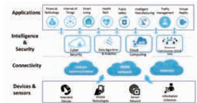
Figure 3: ICT Infrastructure for Smart City Applications
