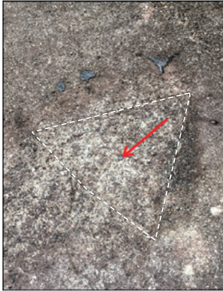
Close-up of the benchmark showing the iron nail marking the centre and the roughly inscribed triangle (today very faint) enclosing it.
