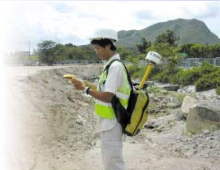
Figure 3 Surveyor with hand-held GPS PDA
